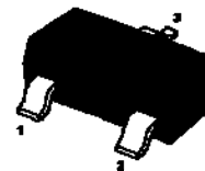
1.Cathode 2.Reference 3.Anode SOT-23 Plastic Package
